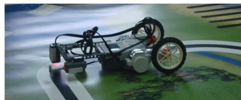
Members programmed their robot to "follow" a black line to reach its destination.
